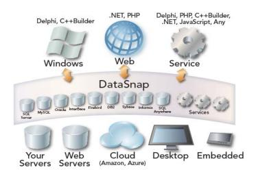
As you can see from the above graphic, DataSnap brings information together with processing and exposure to various client types including Delphi, C++Builder, .NET, PHP, and JavaScript.
